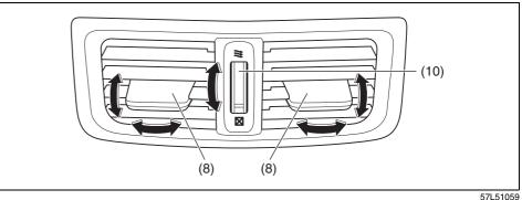
Move the knob (8) vertically or horizontally to adjust the direction of airflow as desired. The center outlet/rear outlet opens when you turn the dial (10) upward and closes when you turn it downward.
